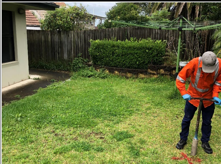
PHOTO 8: HAND AUGER IN REAR OF PROPERTY
